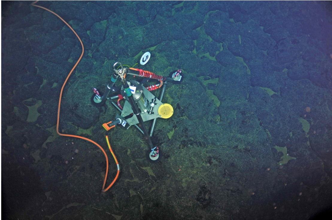
Fig. 4: Combined ocean bottom pressure and tiltmeter mounted on a tripod and deployed at a submarine volcano. Picture from the Ocean Observatories Initiative.
